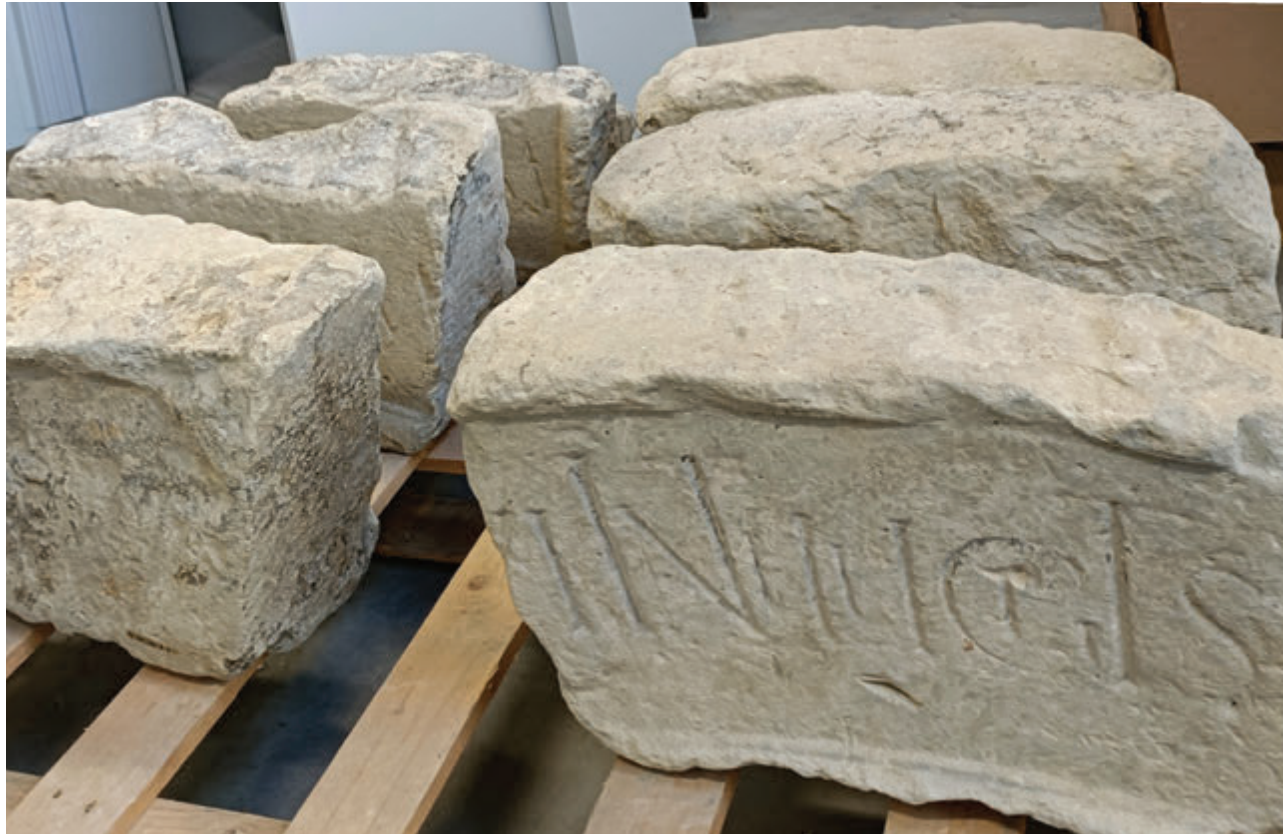
Blocks in Lede stone after a conservation cleaning treatment, forming a former arch at the Maiden's House in Antwerp, Belgium.
