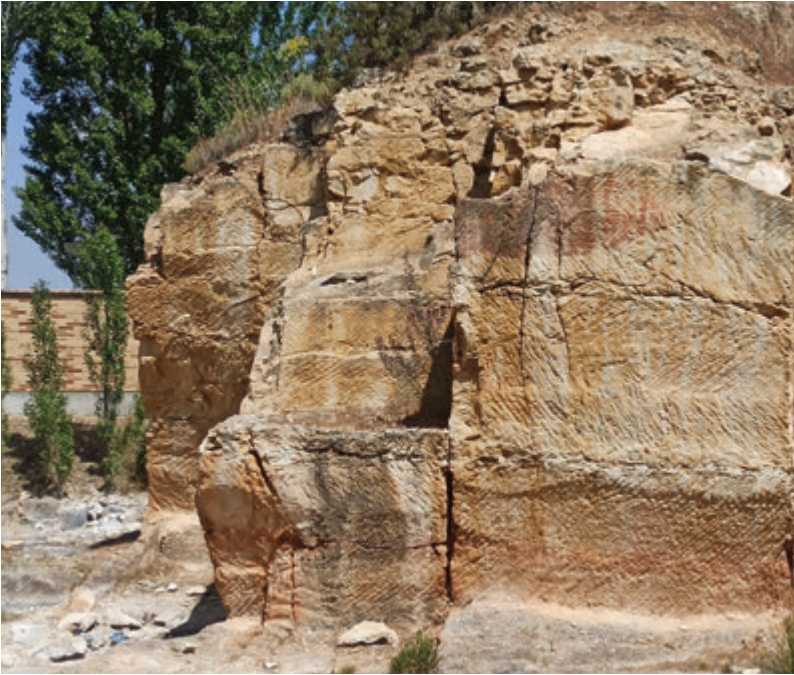
Villamayor Sandstone stonework marks made with the pick, without industrial technology.
