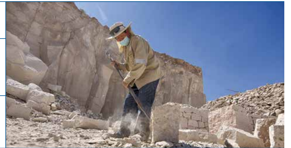
A "Cantero (quarryman)" working to extract sillar in the quarry.
